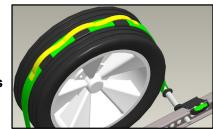
4. Pull strap taut over top of tire and insert cleats into tread keeping the strap centered on the tire. Remove any twists keeping the strap flat with printed text facing up.
